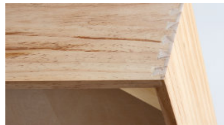
Drawer corner blocks and English dovetailed joints
